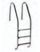
Top Double tread in accordance with BS EN 13451, ladder width 500 mm. Handrails in hand polished Stainless Steel (Ø 43 mm). Treads and rails in Stainless Steel AISI-316. Complete with fixing anchors and earth connection.
