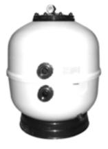
White laminated polyester and fibreglass filter. Internal parts with special sides for OC-1 media. Filter for side selector valve. ¼" air and water purge. Transparent lid with screws. Maximum temperature: 50 °C. Maximum working pressure of 2.5 kg/cm². Maximum filtration speed 50/h/m². Filter for OC-1 filtration media Not compatible with sand, glass or other filter loads. OC1 not included.
